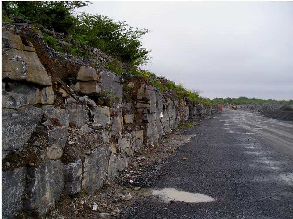
*Plate 2. Epikarst limestone on western side of quarry. Face is developed along a north / south vertical joint.*
