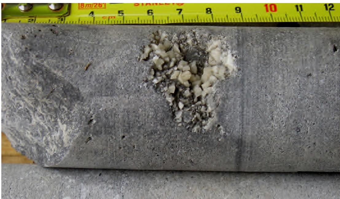
*Plate 10. Vuggy dolomitised interval at 27.4m in Cong A. Note the dolomite crystals lining the vug.*
